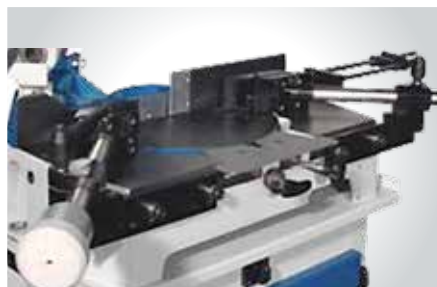
Double horizontal clamps: 45° mechanical with foot-pedal 45° pneumatic with foot-pedal 90° pneumatic with lever
