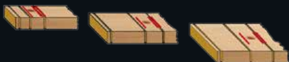
WITH WIDTH SCANNER: Automatic changing of cutting list according to the width.
