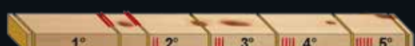
WITH SECOND HORIZONTAL READING CAMERA Cutting lists on five grades by marking on face and edge.
